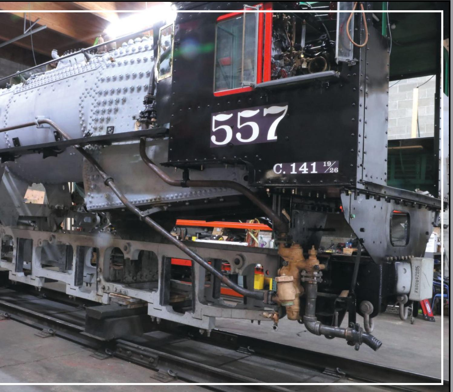
A large portion of the restoration to Locomotive 557 has been completed over an eight-year span. As of December 2019, volunteers continue to work on the boiler while they wait for driving boxes and bearings to return from the Lower 48. (PHOTO COURTESY PAUL DALLESKA)
